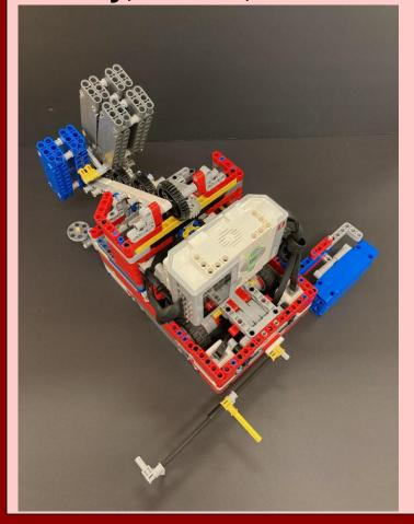
In the last zone, our robot pushes the hinged blue container to the gray circle, drags the airplane and the their truck to destinations, unloads ship, cargo the food separates from the package helicopter, pushes the train to the latch at the end of the tracks, balances the cargo on the ship's west deck, and knocks down the yellow accidentavoidance panel.
